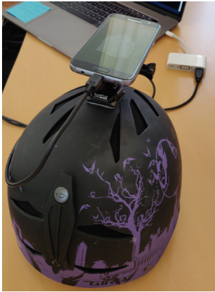
Figure 1: In this image, the android phone is attached on the top of the ski helmet.
